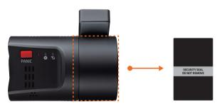
NOTE: IF THE SECURITY SEAL IS REMOVED. THE SEAL WILL DISPLAY 'VOID/OPEN'. SUGGESTING THAT THE CAMERA MAY HAVE BEEN TAMPERED WITH.
