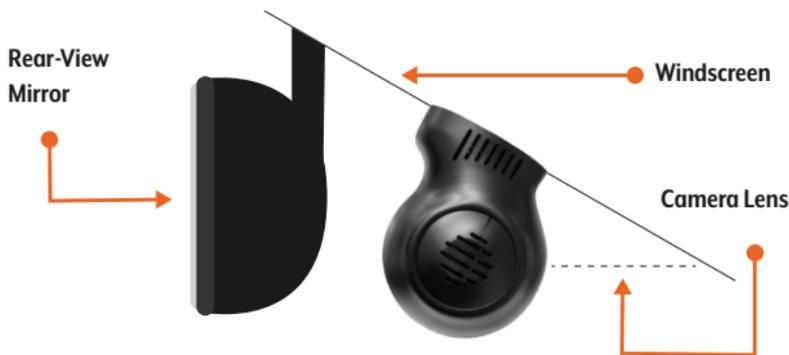
**DO NOT APPLY CAMERA TO TINTED WINDSCREEN SURROUND. MUST BE STUCK TO CLEAR GLASS TO AVOID ANY GPS SIGNAL INTERFERENCE.**
