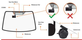
DO NOT APPLY CAMERA TO TINTED WINDSCREEN SURROUND. MUST BE STUCK TO CLEAR GLASS TO AVOID ANY GPS SIGNAL INTERFERENCE.
