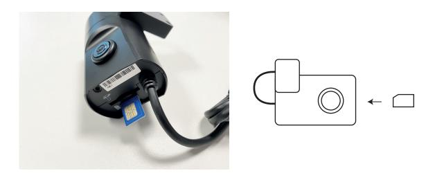
Push until you hear a click, this means the SIM card is in securely, it will also sit flush within the casing. To remove the SIM card, simply push to release.
