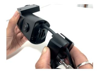
Push SIM card into slot as shown below.
