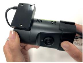
You can now take the key and lock the case, moving the key anti clock-wise. Once complete, please power the camera to confirm SIM Card is being detected. After the camera has booted, you should see BLUE (Recording) + GREEN (Network) lights.
