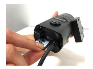
Push the new SD card into the VT2000 until you hear a click, this means the SD card is in securely, it will also sit flush within the casing.
