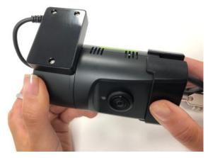
You can now take the key and lock the case, moving the key anti clock wise. once complete please power the camera to confirm the SD card is being detected.
