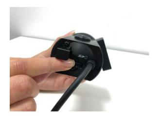
Pull the SD card out of the VT2000 and put this aside.
