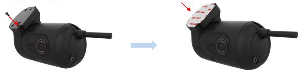
Secure the VT2.2 to the windscreen behind the rear view mirror, <u>below the AS1 line</u>. The camera lens should be as high on the windshield as possible, but still within the windshield wiper zone.
